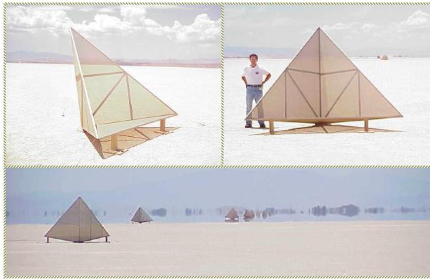
Figure 8: Standard AIRSAR calibration site: the corner reflector array at the Rosamond dry lake bed. Upper left: the corner reflectors are guyed down to keep them stable. The ground is very smooth at radar wavelengths, making for a dark background to the bright corner reflectors. Upper right: the AIRSAR Engineer, Walter Skotnicki poses next to a corner reflector to give a sense of scale. Lower image: several of the reflectors in the array can be seen.
