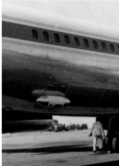
Figure 2. The Rocket Radar antenna adapted to the mounting on the baggage door of the CV990 NASA 711
