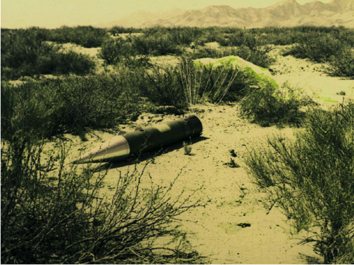
Figure x. The Rocket Radar after the flight. It was recovered by the recovery crew which included Al Laderman and returned to the Navy Lab where post flight calibration was conducted. The radar antenna and camera aperture can be seen facing upwards.
