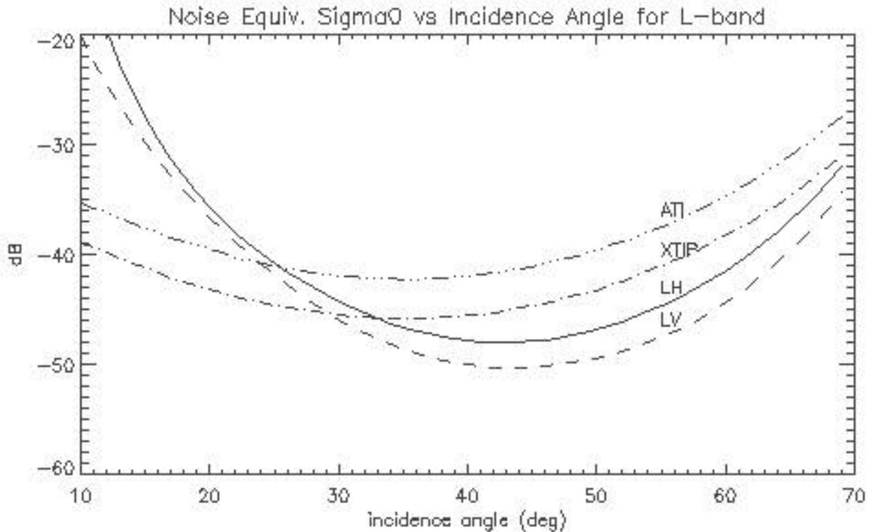
Figure 3. Noise Equivalent Sigma-0 versus incidence angle for CH, CV channels in the POLSAR mode and for ATI, XTI, and XTIP modes assuming 40 MHz chirp bandwidth.
