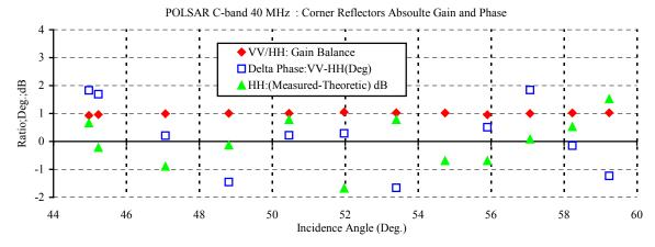
From the above plot, the x-axis indicates incidence angles and y-axis is the CO-POL gain balance ratio, CO-POL phase difference, and an absolute gain of HH channel. Each red diamond represents the VV/HH gain ratio. The
